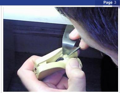
Separate mold and remove model
