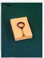
Place rubber moulds into mould frames.
