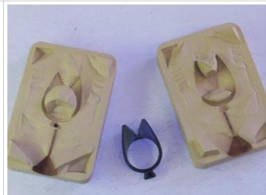
Place on standard wax injector inject wax and allow to cool for up to 15 minutes on heavy sections.
